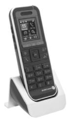
Put your phone on its support. Plug the USB cable into the 5V socket of the desk support. Plug the other end of the USB cable into the AC/DC adapter. Plug the adapor into the mains power supply.
